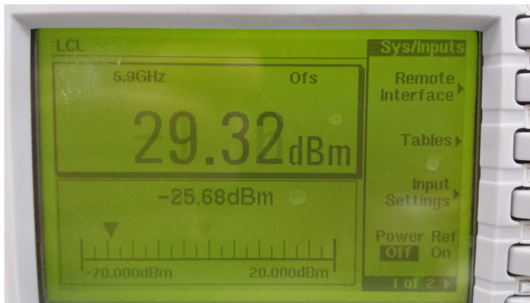
Figure 22. Power Reading from the LGR on an Agilent E4418B Power Meter using a 5 dB attenuator.
